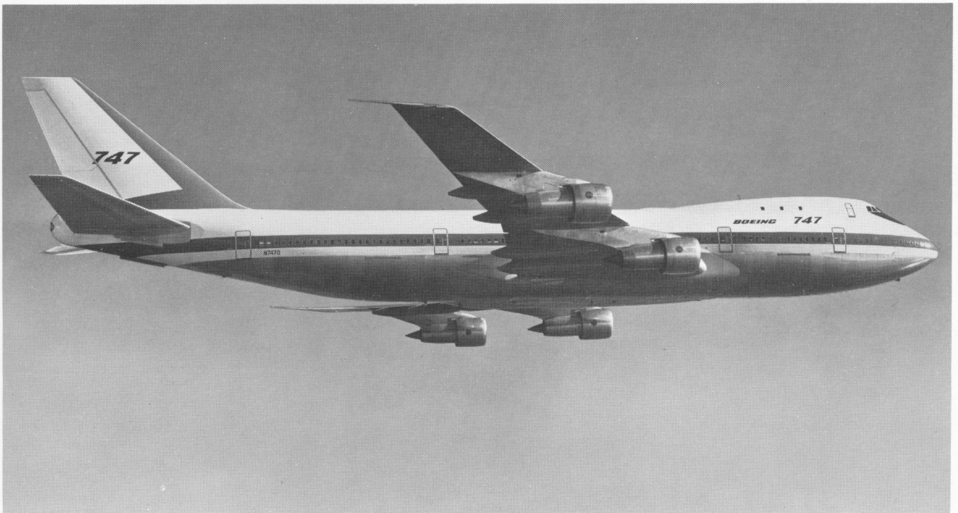
Boeing 747 superjet, winner of Collier Trophy as aviation event of the year, has carried 15 million passengers flying for 26 airlines. Freighter version, ready soon for its first flight, can carry 125 tons of cargo.
